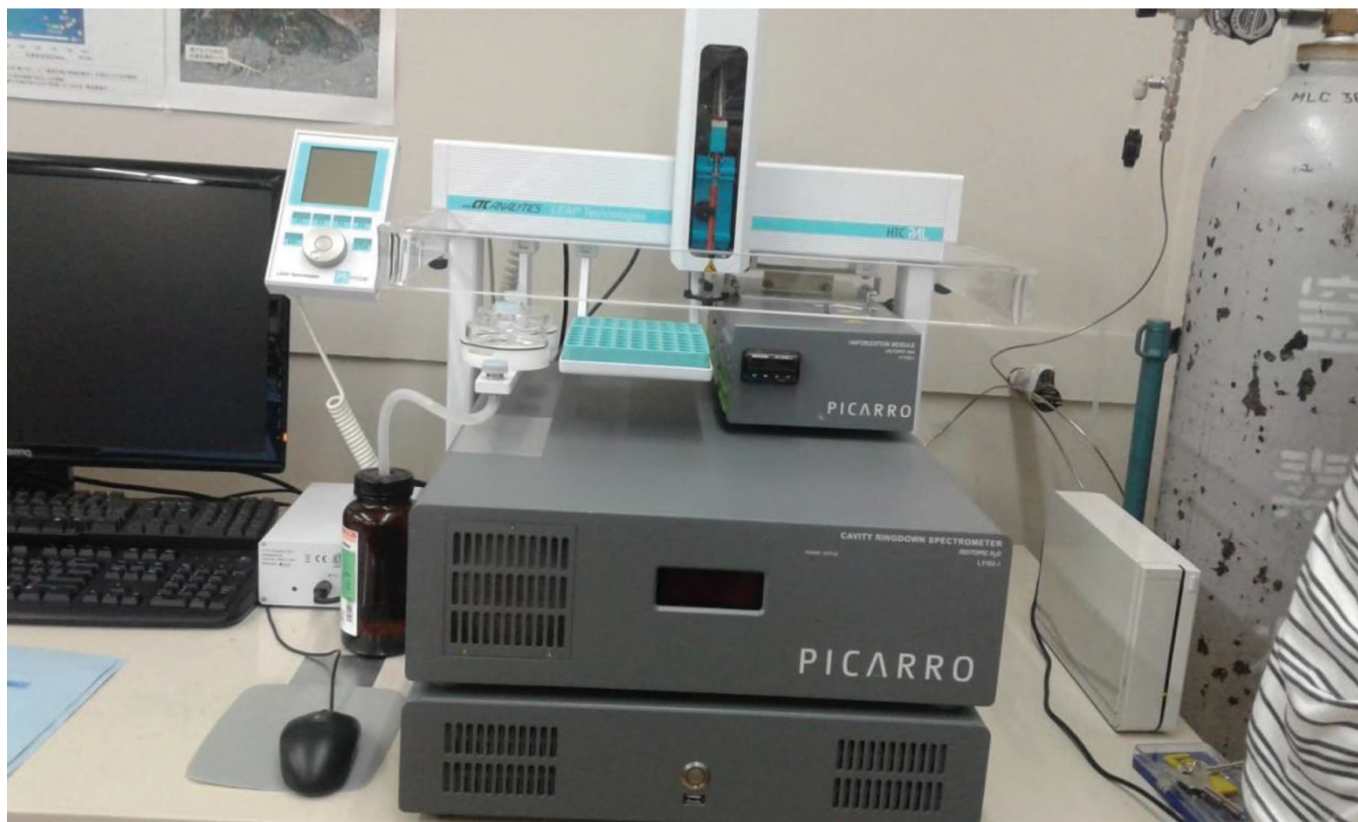
Fig. 1: Instrument of isotope analysis, mass spectrometer (IRMS)
