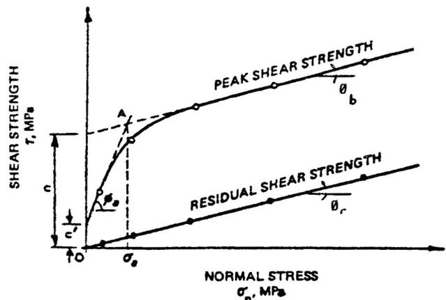
**Fig. 4: Idealized Mohr Coulomb Failure Envelop (theoretical) (IS: 7746, 1991)**
