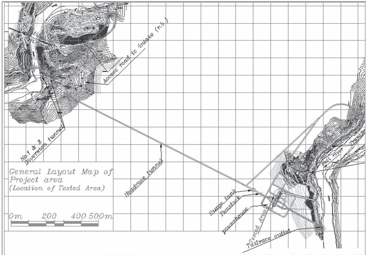
**Fig. 1: Location of tested area at general layout map of Tanahu Hydropower Project (SRCL, 2012; OYO Corporation, 2012)**
