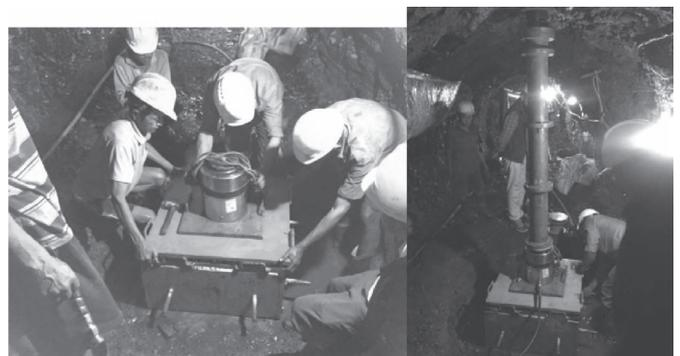
**Fig. 3: Setup the Block Shear Test Machine (ATES, 2017)**
