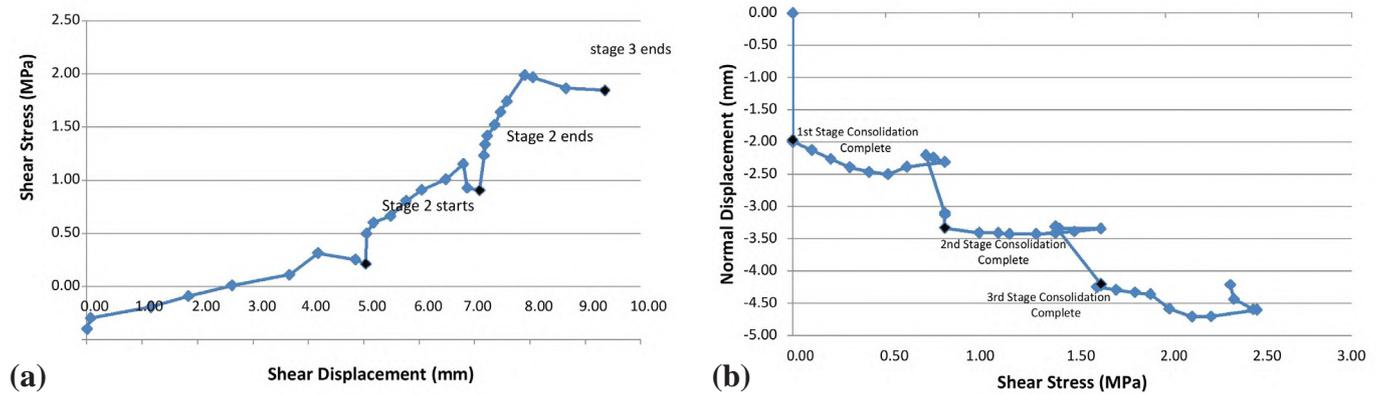
**Fig. 5: (a) Shear stress vs. shear displacement curves for block no. 02 and (b) Shear stress vs. normal displacement curves for block no. 02**
