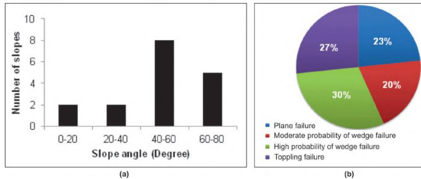
**Fig. 6: Rock slope stability (a) in terms of slope angle and (b) modes of failure probability**
