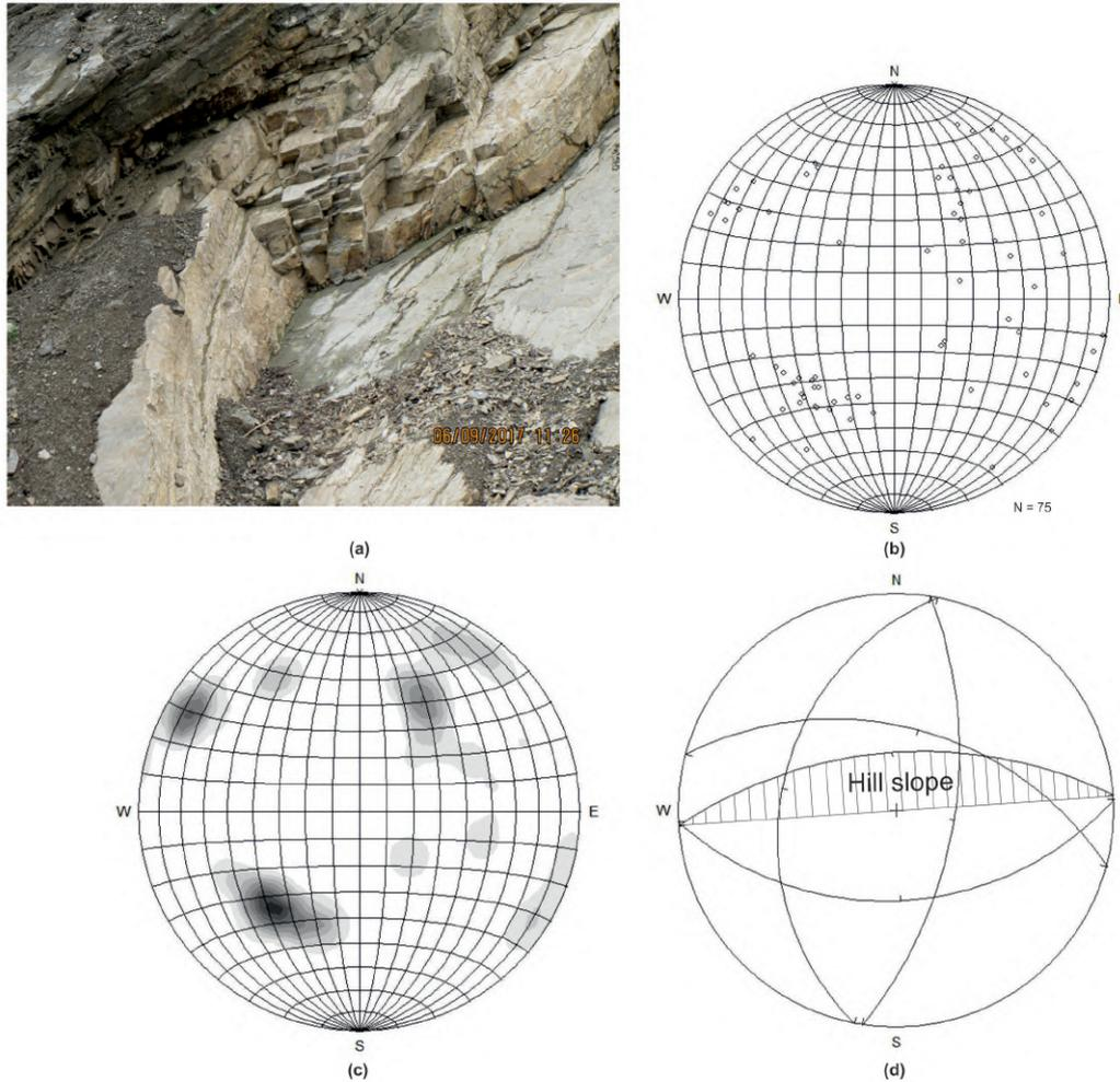
**Fig. 5: Rock-slope stability analysis at Khanigaon (a) slope-face of rock outcrop (b) distribution of major discontinuity poles (c) density stereo-plot of major discontinuities (d) hill-slope and orientation of joints**
